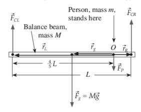
Note that by Newton's third law, the contact force  $\vec{F}_P$  that the person exerts on the beam is equal in magnitude to the upward force that the beam exerts on the person, which (by Newton's *second* law) must be equal in magnitude to the gravitational force  $m\vec{g}$  exerted on the person (assuming the person its at rest).
