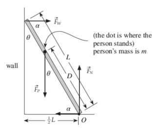
The force  $\vec{F}_P$  that the person exerts on the ladder must by Newton's third law be equal in magnitude to the force that the ladder exerts upward on the person. If the person is not moving, then this upward force must cancel the downward force of gravity on the person. This chain of reasoning therefore implies that  $|\vec{F}_P| = m|\vec{g}|$ , where m is the person's mass. If we ignore the ladder's mass, then Newton's second law for the ladder states that
