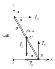
(The static friction force points in the -x direction from point B.)
