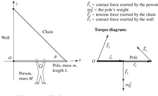
**Known:**  $|\vec{r}_2| = L = 1.8 \text{ m}, |\vec{r}_1| = \frac{1}{2}L, M = 65 \text{ kg}, m = 8 \text{ kg}, \theta = 45^{\circ}$ **Unknown:**  $|\vec{F}_1| = ? |\vec{F}_2| = ? \vec{F}_3 = ?$
