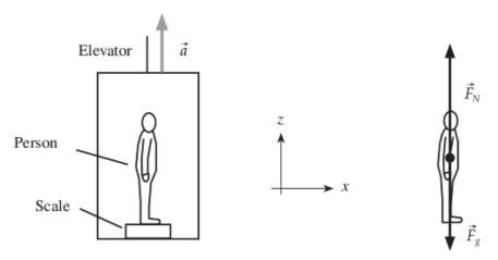
As discussed in example N5.5, the scale reads the magnitude of the normal force that it exerts on the person. Since the person is accelerating (along with the elevator) relative to the building frame (which we will take to be inertial) in such a way that  $a_z = 1.8 \text{ m/s}^2$ , the z component of Newton's second law implies that  $|\vec{F}_N| - |\vec{F}_g| = ma_z$ , which we can solve for  $|\vec{F}_g|$ . Doing this yields
