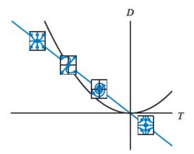
(b) The trace T is 2a, and the determinant D is -a. Therefore, the curve in the trace-determinant plane is D = -T/2. This line crosses the parabola  $T^2 - 4D = 0$  at two points—at (T, D) = (0, 0) if a = 0 and at (T, D) = (-2, 1) if a = -1.
