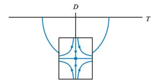
(b) The curve in the trace-determinant plane is the portion of the unit circle centered at 0 that lies in the half-plane  $y \le 0$ .
